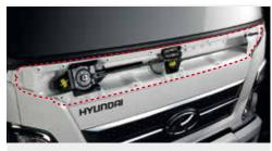
**Detachable upper front panel** The detachable design allows for quick inspections and easier servicing.
