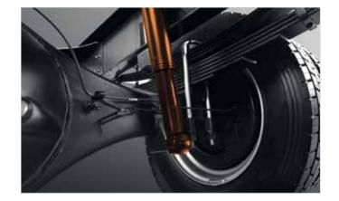
**Improved Rear Suspension** New rubber dampers replace the older metal-type to deliver greatly improved rear suspension performance.
