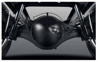
**Anti–Vibration Dampers** Vibration has been reduced by the application of gas–type shock absorbers and wider spacing between the leaf springs.
